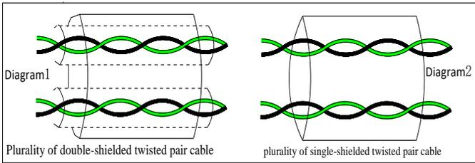
For low-voltage digital signals, double-shielded cable is the best choice, but can also be a single-shielded or unshielded twisted pair, as shown in Figure 2, however, the frequency of the signal, it can only use a shielded cable.
