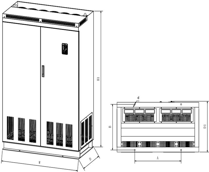
Figure 7-9: 450kW~630kW G3 (DC reactor) dimension
