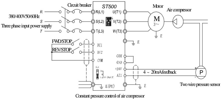
**V-11-2 Connection:** Short circuit between COM and GND;
