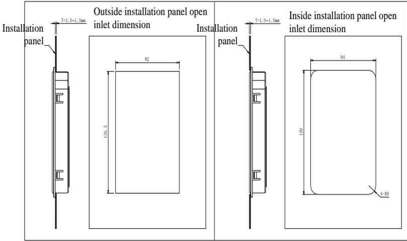
Figure 7-13:ST500 keyboard installation open inlet dimension(mm)
