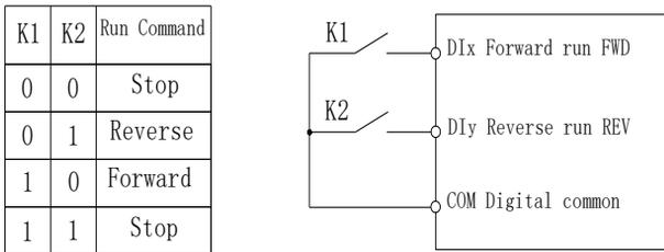
Figure 5-3:Terminal command mode: Two wire mode 1
