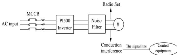
(1) Inductive interference countermeasure : in addition to the installation of noise filter , it can also import the output cables to grounded metal tube. The distance between the output cable and signal line is greater than 30cm , the influence of inductive interference is also significantly reduced. As shown below :
