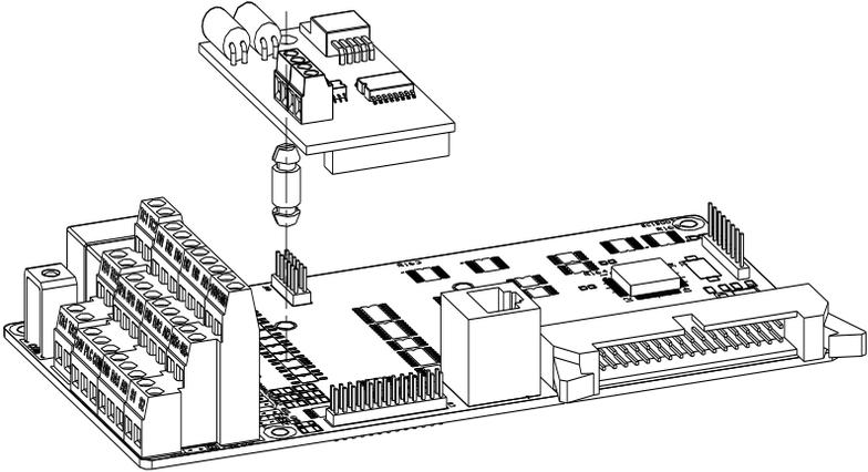
Figure III-1: CAN bus communication card's installation on SCB
