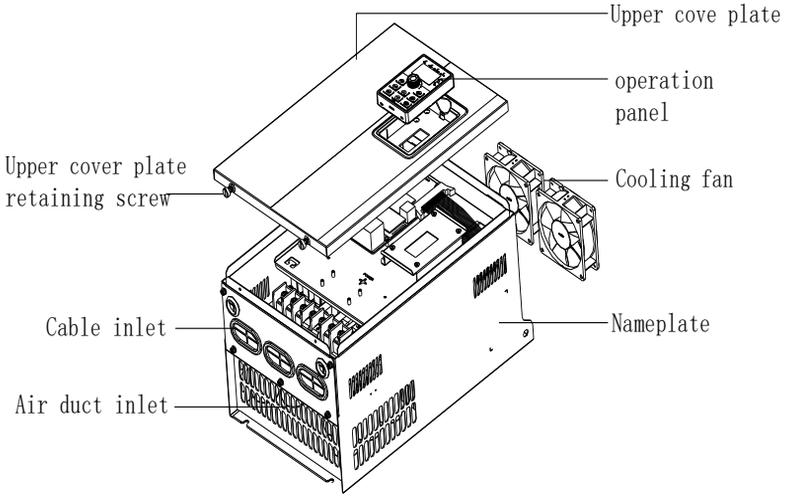
Figure 7-1: Product outside drawing (15kW G3), installation dimension
