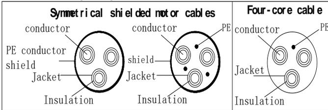
Note: If conductivity of the cable shield can not meet the requirements, you must use a separate PE conductor.
