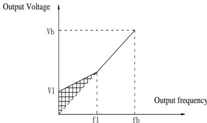
V1: Manual torque boost voltage Vb: Maximum output voltage
