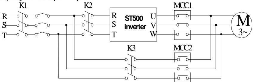
MCC1 & MCC2 interlocking AC contactor
