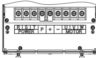
Figure 4-8: 30kW~37kW G3 main circuit terminal
