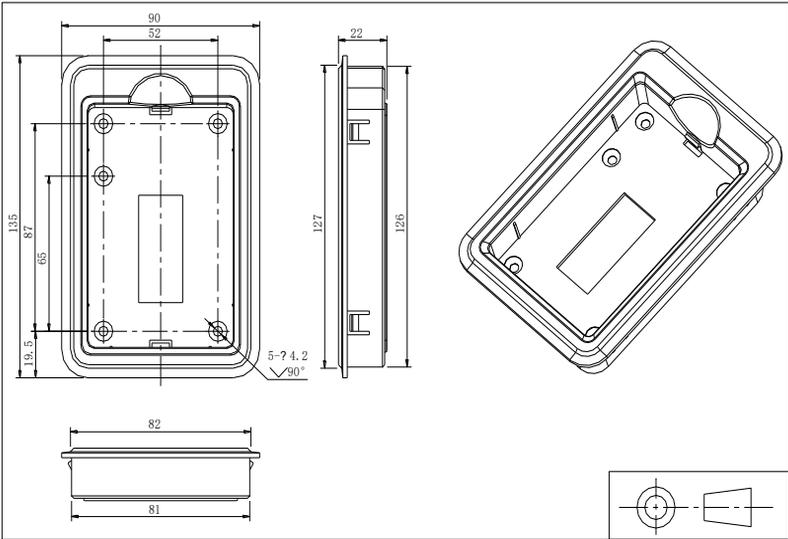
Figure 7-12:ST500 Keyboard dimension (mm)
