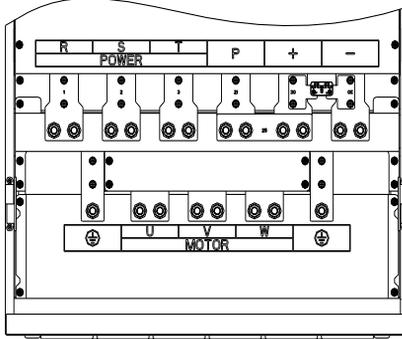
Figure 4-13: 250kW~400kW G3 main circuit terminal
