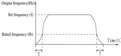
Figure 5-11:Schematic diagram of S curve ac/deceleration B
