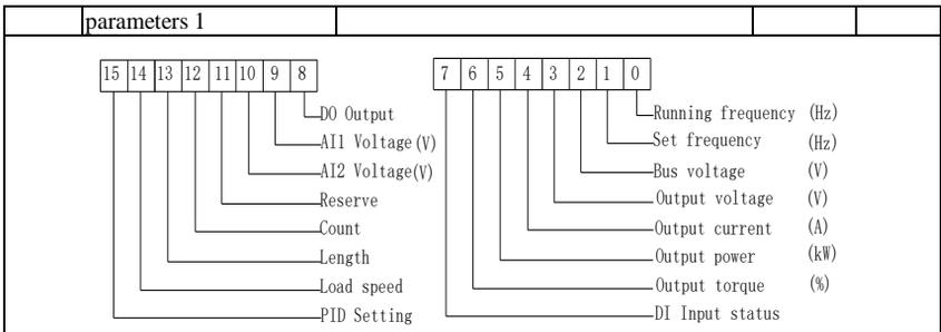
Figure 5-15: The figure is the Running status 1
