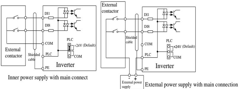
Figure 4-16: Signal input terminal circuit, dry contact mode
