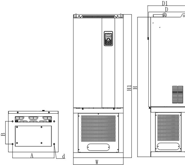
Figure 7-7: 160kW~220kW G3 (Base with DC reactor) Outline dimension
