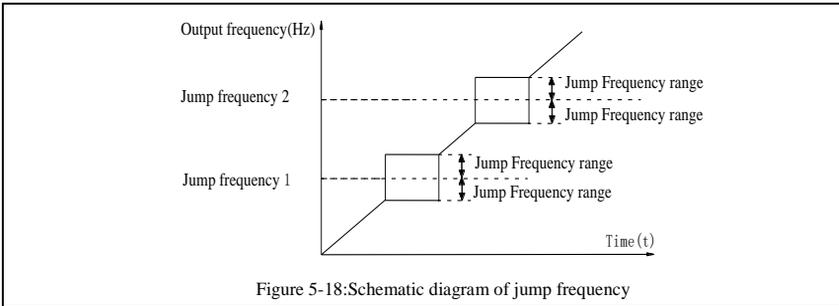
Figure 5-18:Schematic diagram of jump frequency
