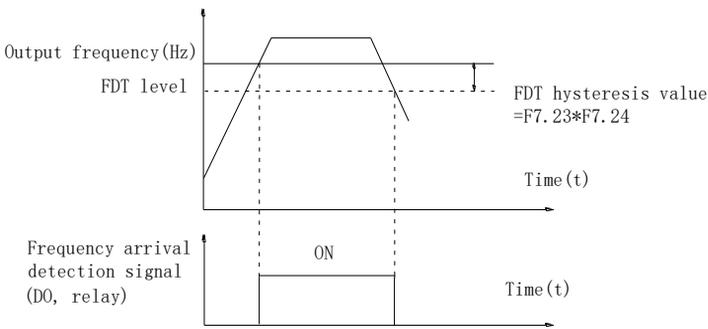
Figure 5-22:Schematic diagram of FDT level
