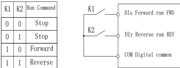
Figure 5-4:Terminal command mode: Two wire mode 2
