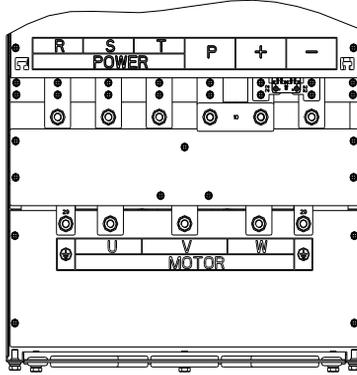
Figure 4-12: 160kW~220kW G3 main circuit terminal
