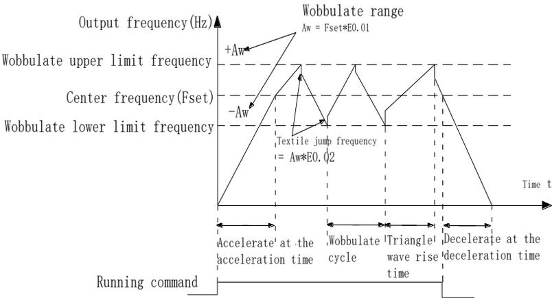
Figure 5-29:Schematic diagram of wobble operating
