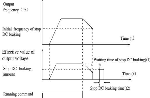
Figure 5-9: Schematic diagram of stop DC braking time
