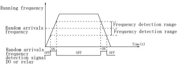
Figure 5-24:Schematic diagram of random arrivals frequency detection
