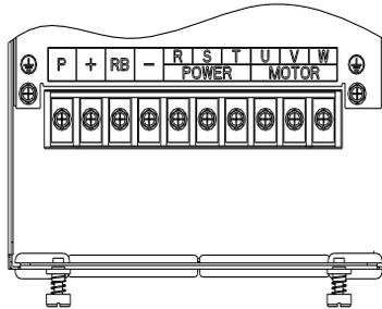
Figure 4-6: 15kW G3 main circuit terminal
