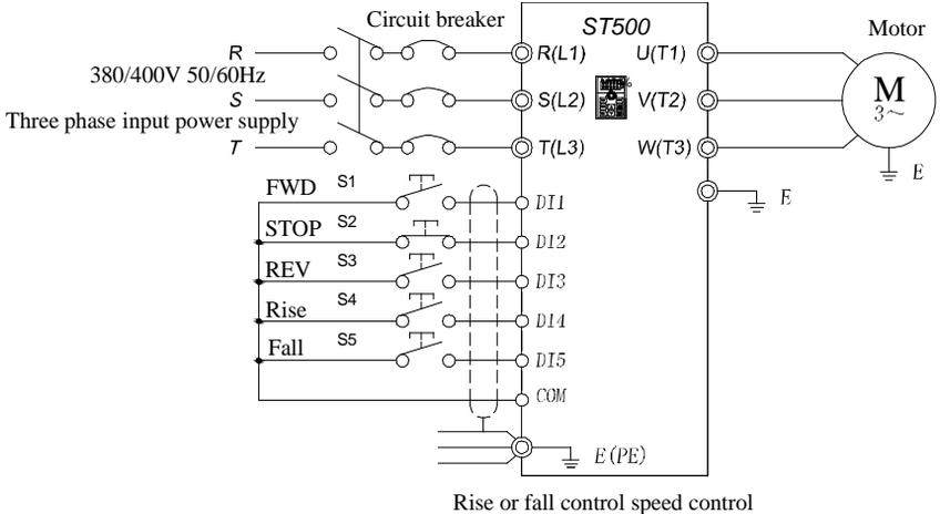
**V-8-2 Connection:** Three-wire control mode 1, forward command Corresponding terminal DI1, stop DI2, reverse DI3, and DI4 and DI5, respectively, with the corresponding COM short, increase and decrease running frequency command.
