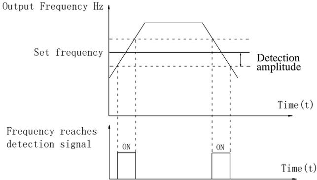
Figure 5-23:Schematic diagram of frequency arrival detection amplitude
