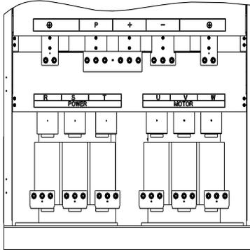
Figure 4-14: 450kW~630kW G3 main circuit terminal
