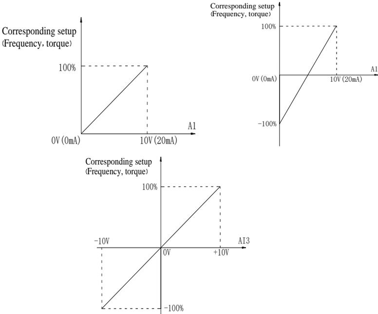
Figure 5-7:Relationship between analog reference and set amount
