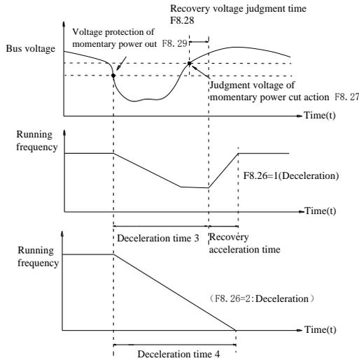
Figure 5-28: Schematic diagram of momentary power cut action
