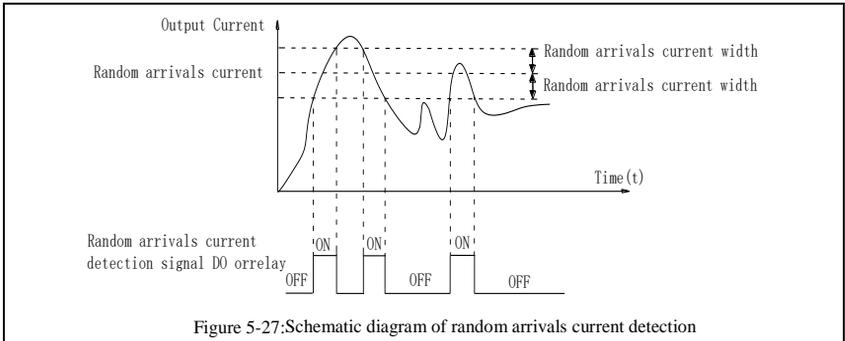
Figure 5-27: Schematic diagram of random arrivals current detection
