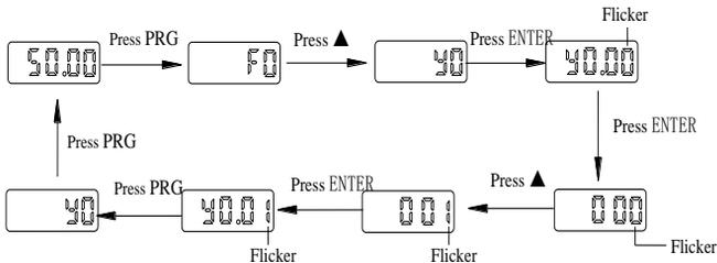
Without blinking digit, the function code can not be modified in the level 3 menu. The reason may be one of the following:
