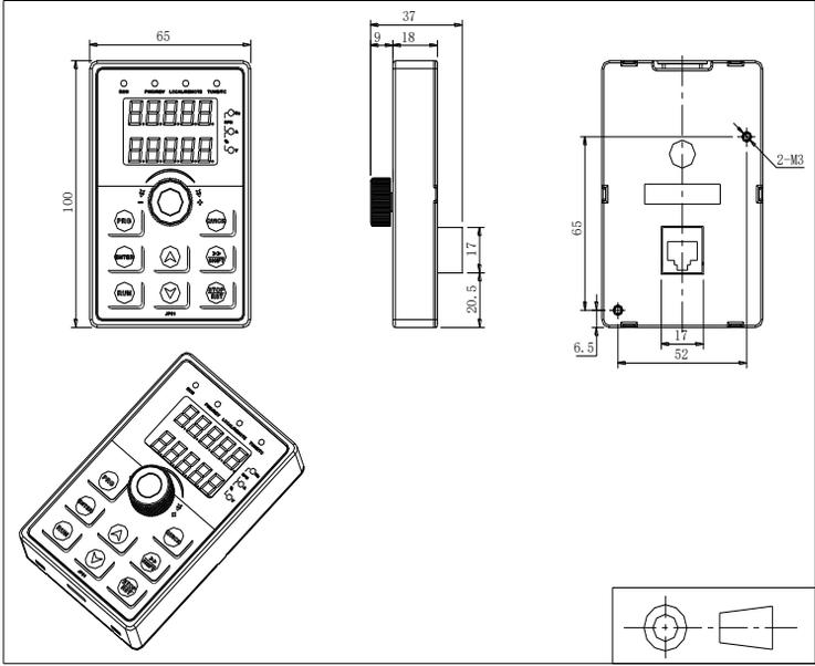
Figure 7-11:ST500 Keyboard dimension (mm)
