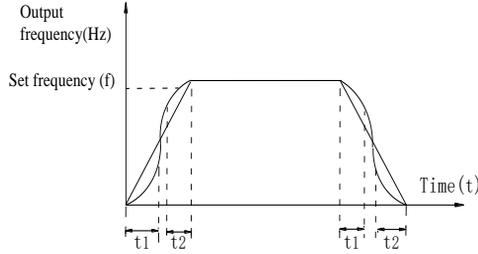
Figure 5-10:Schematic diagram of S curve ac/deceleration A
