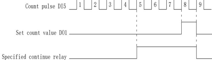
Figure 5-30:Schematic diagram of the set count value reference and the specified value
