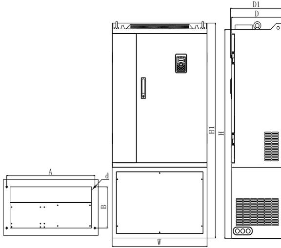
Figure 7-8: 250kW~400kW G3 (Base with DC reactor) Outline dimension
