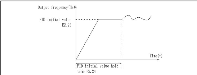
Figure 5-34: functional schematic of PID initial value.
