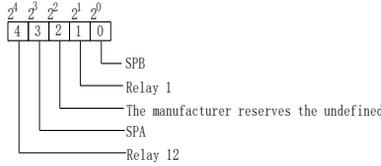
Figure 5-2:DO the sequence of the Output terminal
