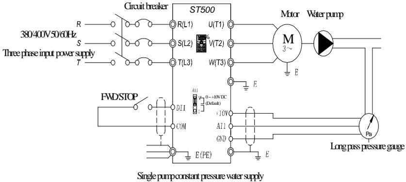
Note: Check the wiring is correct, close the circuit breaker, the inverter power, press the forward button for 1-2 seconds and then stop, check the pump running direction, if the direction is reversed, then change the motor wiring phase sequence
