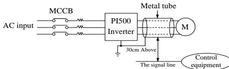
(2) Radio frequency (RF) interference countermeasure: the input cables, output cables and inverter itself can produce interference, to install noise filter on both sides of input and output and shield the inverter with metal box can reduce the radio frequency interference. As shown below :
